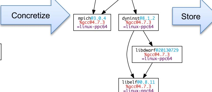
Concrete spec is fully constrained and can be passed to install.
