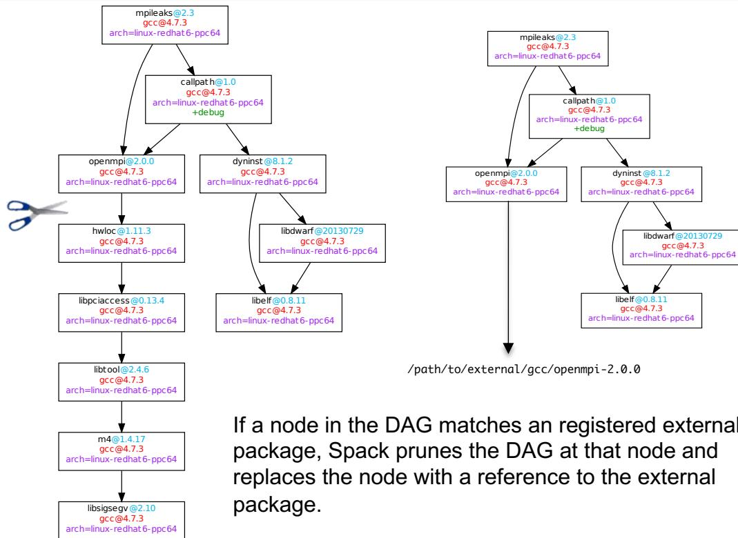
If a node in the DAG matches an registered external package, Spack prunes the DAG at that node and replaces the node with a reference to the external package.
