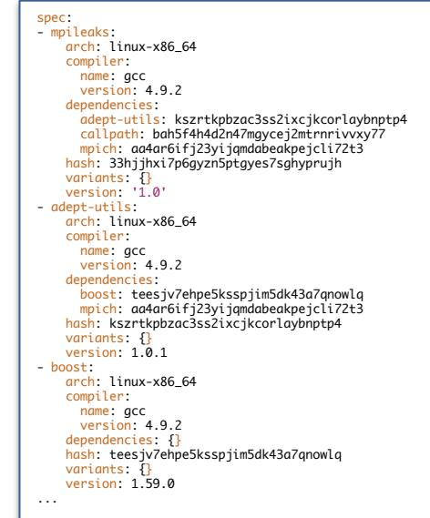
Detailed provenance is stored with the installed package
